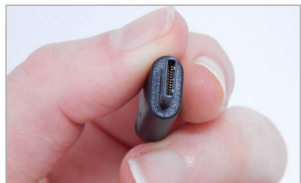
The USB Type C connector can be inserted into Vario 440 in either direction.
