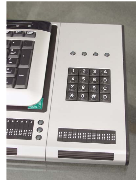
The modules are fitted either to the left or the right side of VarioPro.
